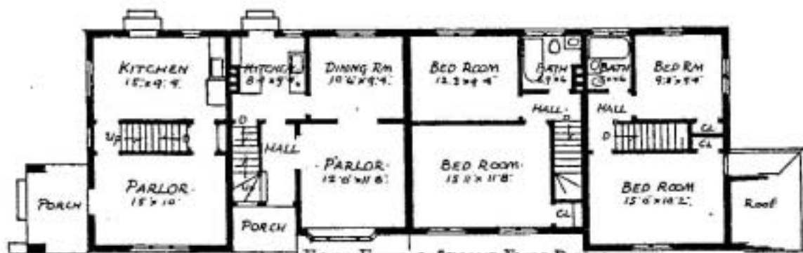
FIRST FLOOR & SECOND FLOOR PLANS Plans of Quadruple Four and Five-Room Houses
